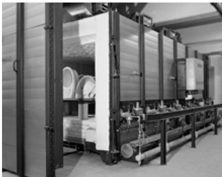
Intermittent shuttle kiln in the ceramics industry
